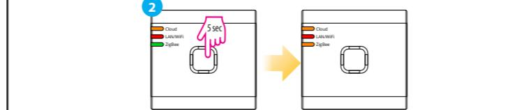
To start the system installation press and hold the button for 5 seconds until ZigBee LED turn solid orange. This means the ZigBee network is ready to accept Salus Premium devices.
