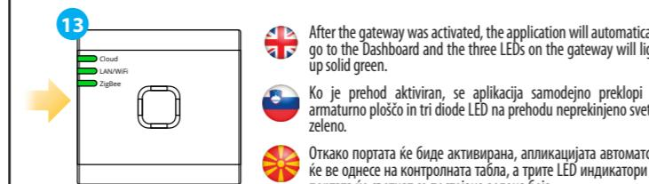
After the gateway was activated, the application will automatically go to the Dashboard and the three LEDs on the gateway will light up solid green.
